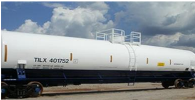
Figure 49. 21,964 gallon non-coiled, insulated car designed to operate at a 286,000 lbs. gross rail load for the transportation of carbon dioxide.
