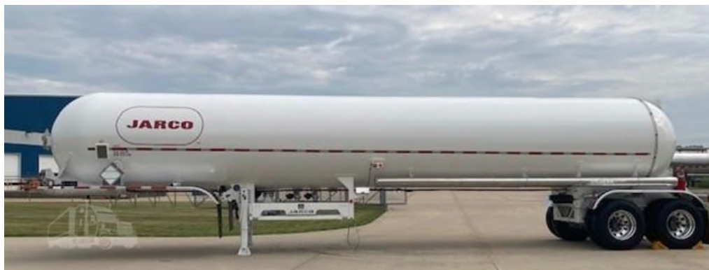
Figure 25. 10,600-gallon, 265 PSI, MC 331 Liquid Tanker
